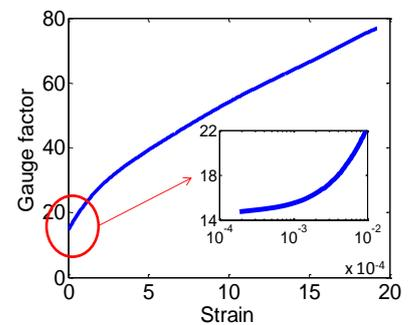
Fig.4 Gauge factor versus strain after mechanical stabilization (25 cycles).
